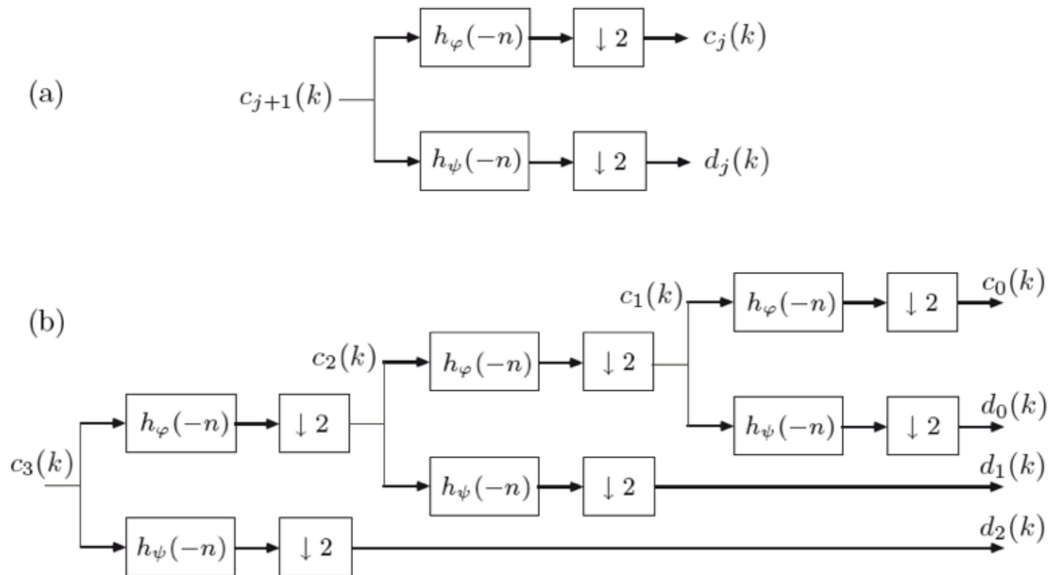
**Figure 4.43:** (a) A two-channel analysis filter bank for calculating the coefficients of the wavelet series expansion in (4.333). (b) The discrete wavelet transform based on the filter bank in (a), which, in this case, produces the coefficients that decompose the space  $\mathcal{V}_3$  into  $\mathcal{V}_0$ ,  $\mathcal{W}_0$ ,  $\mathcal{W}_1$ , and  $\mathcal{W}_2$ .
