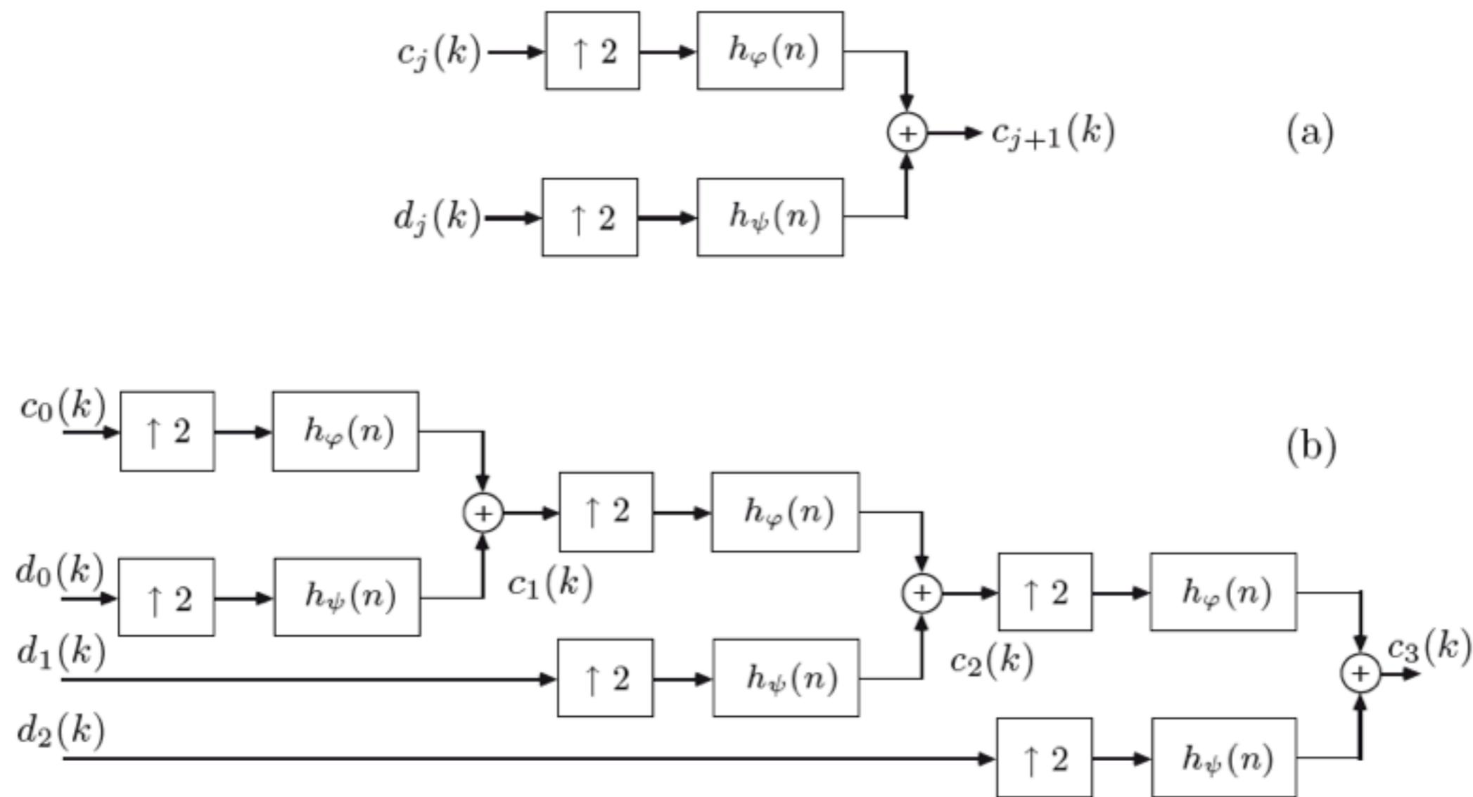
**Figure 4.45:** (a) A two-channel synthesis filter bank. (b) The inverse discrete wavelet transform based on the filter bank in (a) which, in this case, produces the coefficients of the space  $\mathcal{V}_3$  based on  $\mathcal{V}_0, \mathcal{W}_0, \mathcal{W}_1,$  and  $\mathcal{W}_2$ .
